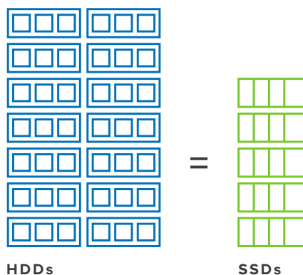
Figure 2 - SSDs can save data center space, at a ratio of approximately 5:2, based on vendor reporting.
